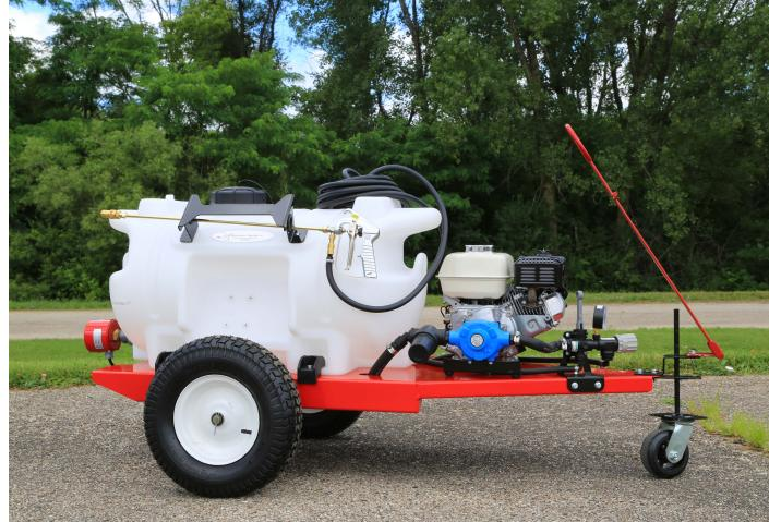
Our gas powered 40 gallon cart is designed for outdoor de-icing operations. This cart uses a 5.5 HP air-cooled gasoline engine, providing adjustable fluid flow rates and pressures of up to 7 GPM/150 PSI, sufficient to de-ice all general aviation, corporate & charter aircraft. The cart is equipped with an electric immersion heater to heat the de-icing fluid to a maximum of 140°F to help melt frost, snow & ice from your aircraft's surfaces.
